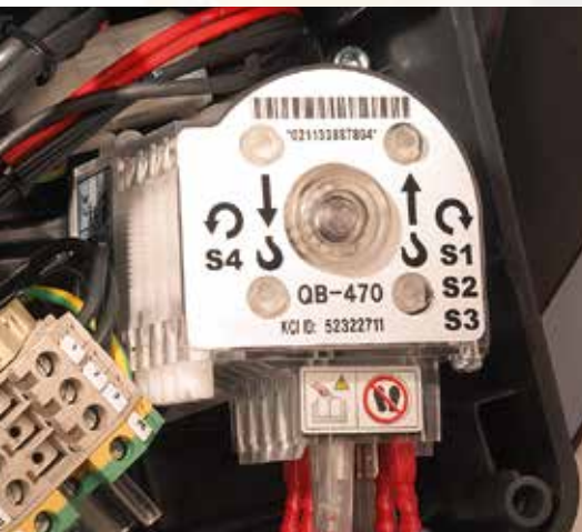
Hoisting gear limit switch
